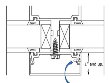
On horizontals, (2) 1/16" X 5/16" Roll Pins need to be located on top side (when possible) of horizontal and place between 1/4 and 1/3 points of D.L.O.
