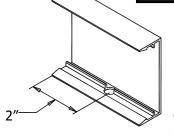
Drill 5/16" diameter weep holes in the horizontal covers at 2" from daylight opening
