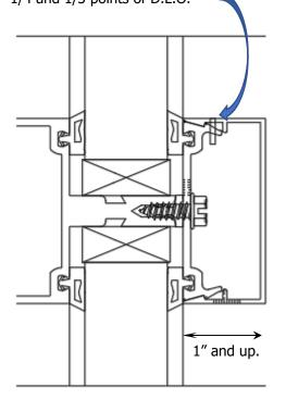
On Verticals, a single 1/16" X 5/16" Roll Pin is to be used in order to prevent vertical slippage and is recommended to be located at center of cover's cut length (or as near as possible) but can be located at a horizontal to eliminate exposure.
